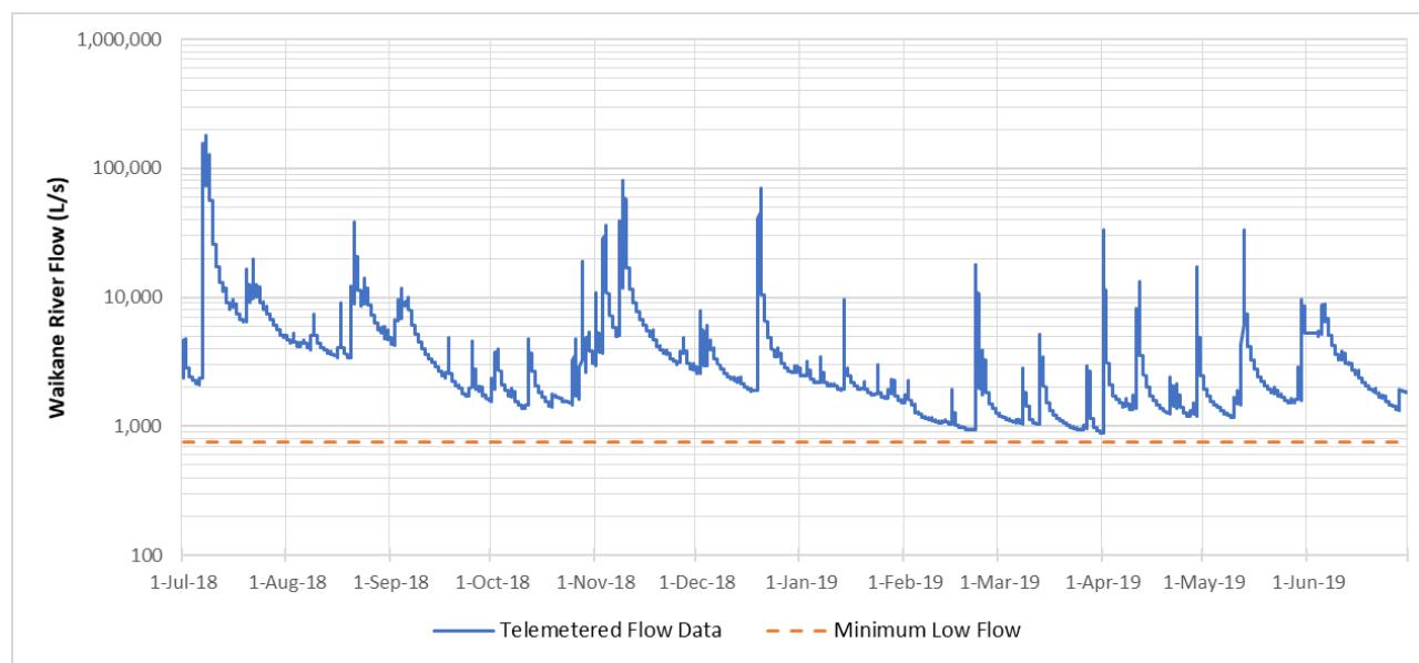
Figure 2: Waikanae River Flow at Water Treatment Plant (July 2018 – June 2019)
