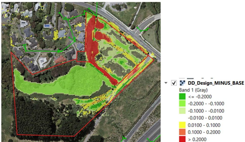
DEPTH DIFFERENCE (DESIGN MINUS BASE) (Red thru Yellow = increase, green = decrease)
