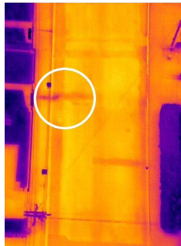
Drone leak detection image in Ōtaki.
