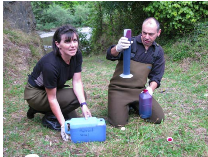
NIWA scientists Janine Wech and Dr Alastair Suren prepare dye for testing Waikanae River flows.
