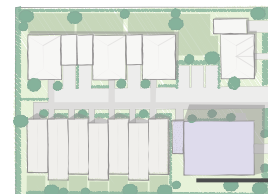
DIAGRAM 14 - LANDSCAPE TREATMENT USED TO SOFTEN HARD EDGES AND IMPROVE OUTLOOK, DIFFERENT CONCRETE MATERIAL DELINEATES PEDESTRIAN AND VEHICULAR SPACES
