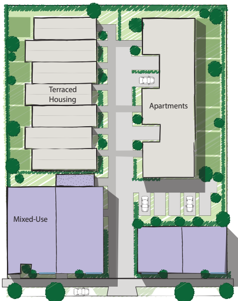
DIAGRAM 16 - LANDSCAPING USED TO SOFTEN HARD EDGES AND IMPROVE OUTLOOK, DIFFERENT CONCRETE MATERIAL DELINEATES PEDESTRIAN AND VEHICULAR SPACES
