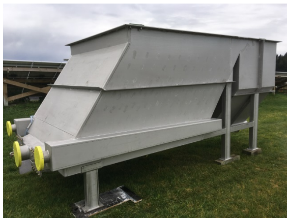
The new dissolved air flotation package plant on site at the Paraparaumu wastewater treatment plant ready for installation
