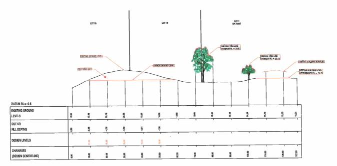
01 EW CROSS SECTION SHT 1 HORIZONTAL SCALE: 1:500 VERTICAL SCALE 1:500
