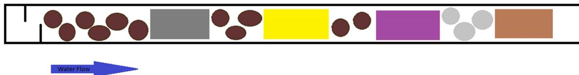
**Figure 2-2: Schematic drawing of channel showing baffles at the head of the channel and the number and layout of substrates.** Pre-colonised river cobbles are dark brown and bare cobbles (no periphyton) are light grey. Rectangles show type and location of artificial substrates: tiles (grey rectangle), Styrofoam (yellow), felted substrate (pink) and brick paver (light brown). Blue arrow indicates direction of water flow.
