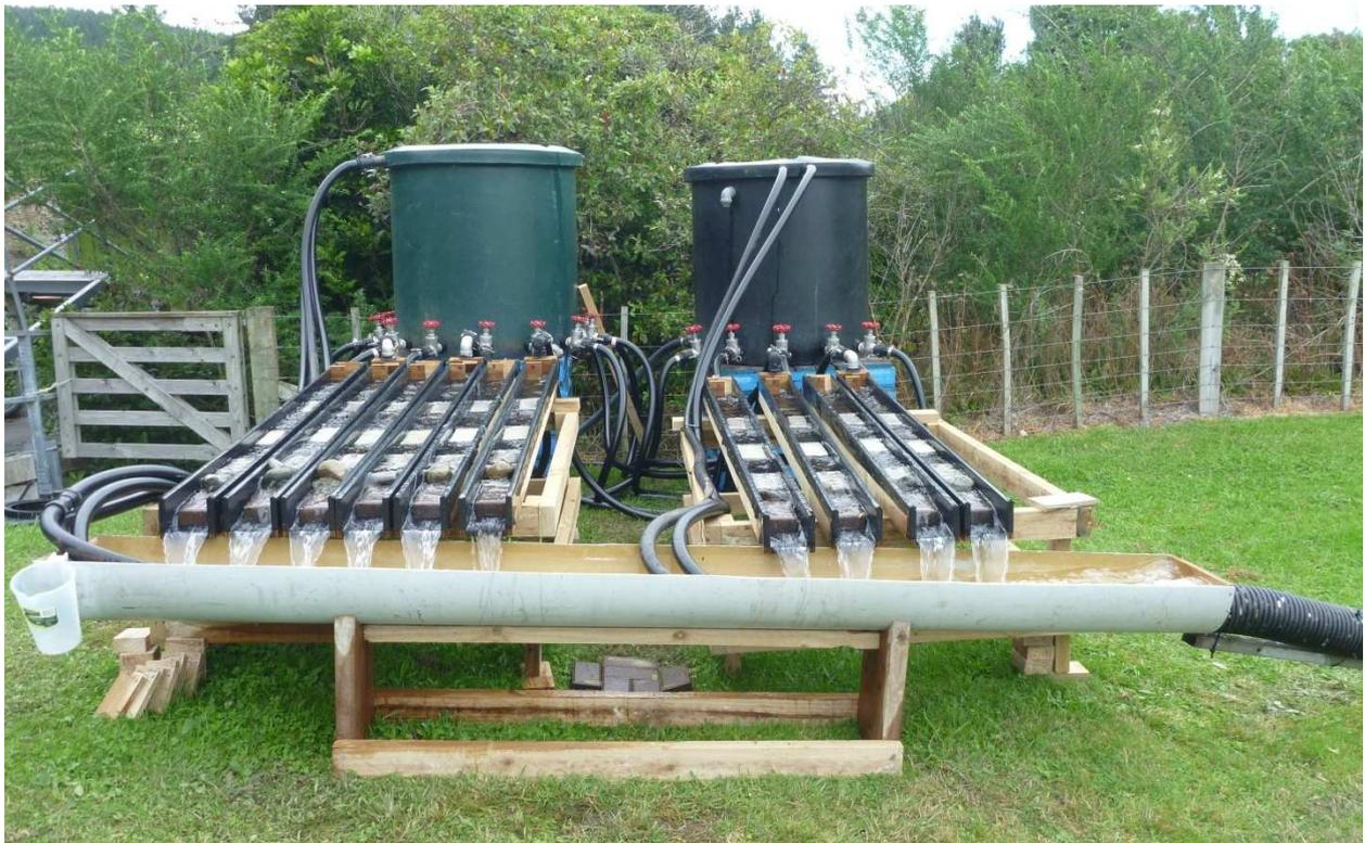
**Figure 2-1: Experimental set-up showing layout of water supply tanks and channels (Day 1).** Substrate layout and water flow are similar for all channels. Water drains into single large channel and returned to the Waikanae River.
