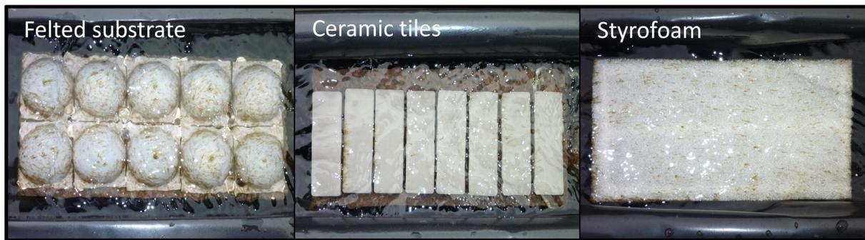
**Figure 2-3: Artificial substrates in-situ on Day 1 of the experiment.** Total depth of felted substrate was 70mm; ceramic tiles 60 mm; and Styrofoam 55 mm.
