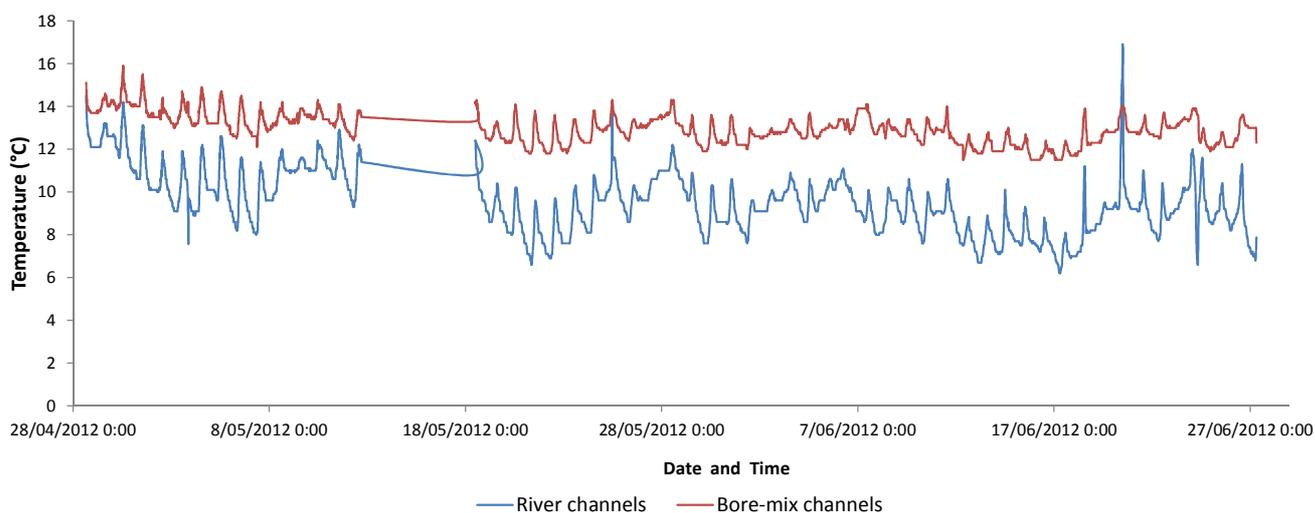
**Figure 3-1: Temperature in river and bore-mix channels.** Temperature spikes in river channels on 25 May and 20 June correspond to low water levels in the river water supply tank. Straight lines for both river and bore-mix temperature data between 12 and 18 May indicate temperature logger failure.
