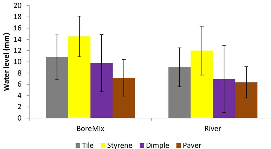
**Figure 3-2: Mean water level flowing over artificial substrates in river and bore mix channels.** Error bars show standard deviation.
