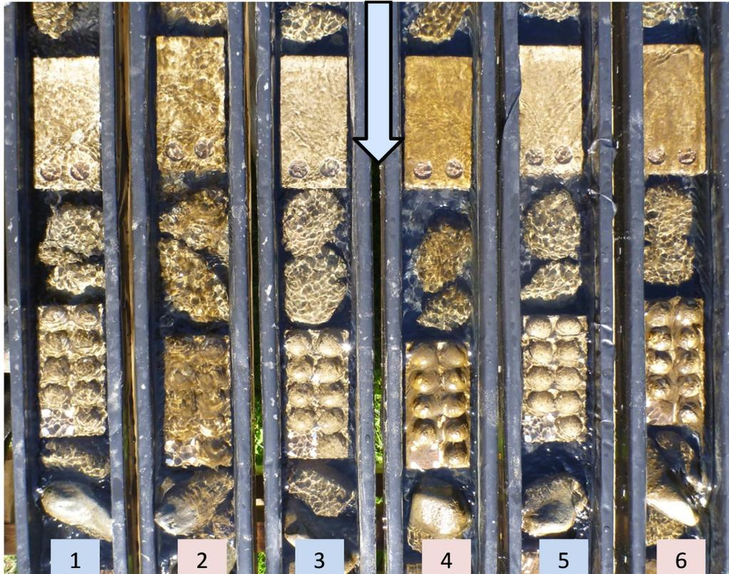
**Figure 3-3: Section of Channels 1 to 6 after sampling event at Day 19.** Styrofoam substrates are at top of photo and felted substrates are near bottom of photo. River cobbles are interspersed throughout channels. River channels are 1, 3 and 5; Bore-mix channels are 2, 4 and 6. Arrow shows direction of water flow. Khaki-green filamentous periphyton is clearly seen in bore-mix channels.
