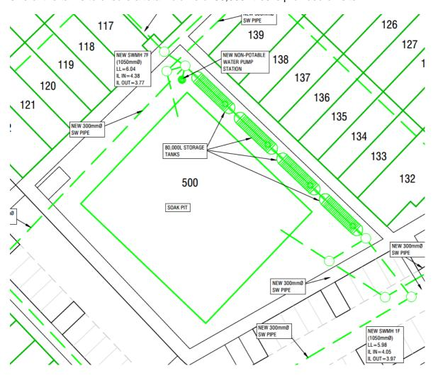
The tanks are proposed to be filled by the roof water only from Lots 1-23 and 37-139. The roof area from Lots 24-36 and the roading network will be directed into the soakage system. The overflow from the tanks will be connected to the proposed soakage system. A stormwater pump will be provided to get water out of the tanks and into an irrigation system and to provide water to the refuse areas.
