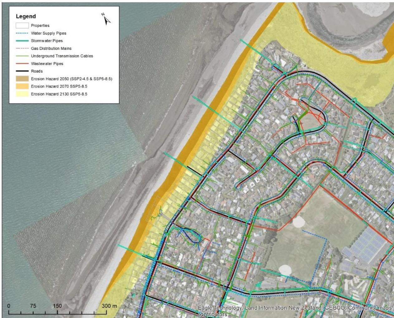
Figure 3.3: Key infrastructure around the Manly Street Area potentially impacted by coastal erosion.
