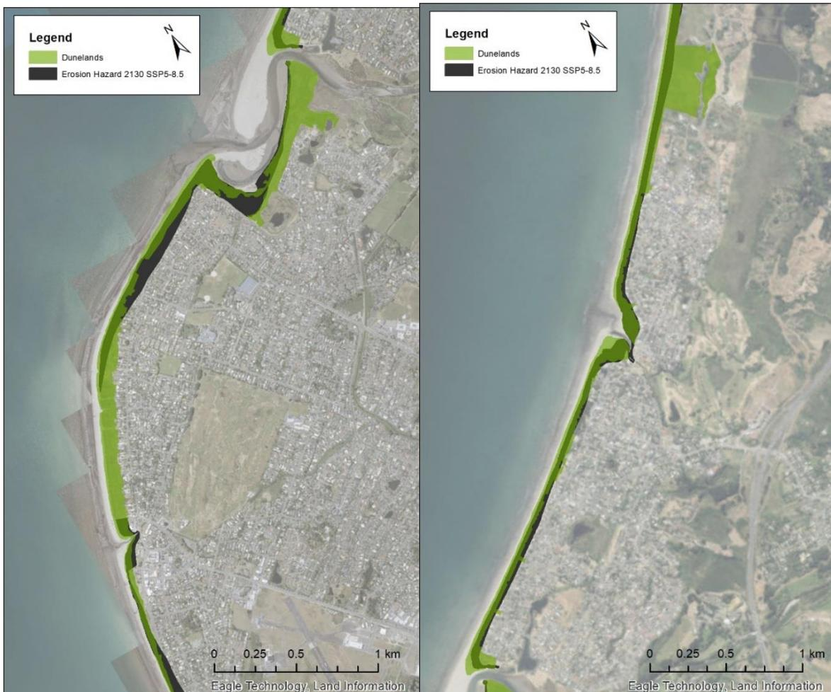
Figure A.3.1: Exposure of the dunelands to erosion hazards in 2130 under SLR scenario SSP5-8.5.
