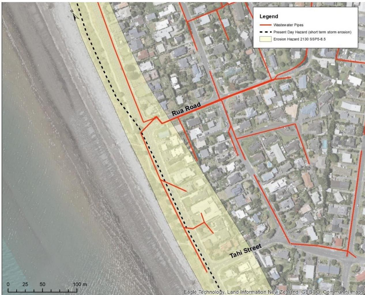
Figure 3.4: Wastewater network pipes southern Paraparaumu potentially impacted from the short-term storm hazard at present sea levels.
