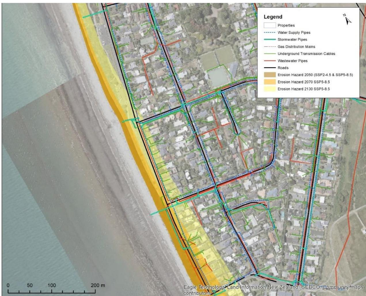
Figure 3.2: Infrastructure network impacted by projected future coastal erosion at the southern end of Marine Parade.
