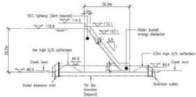
SPILLWAY CROSS SECTION
