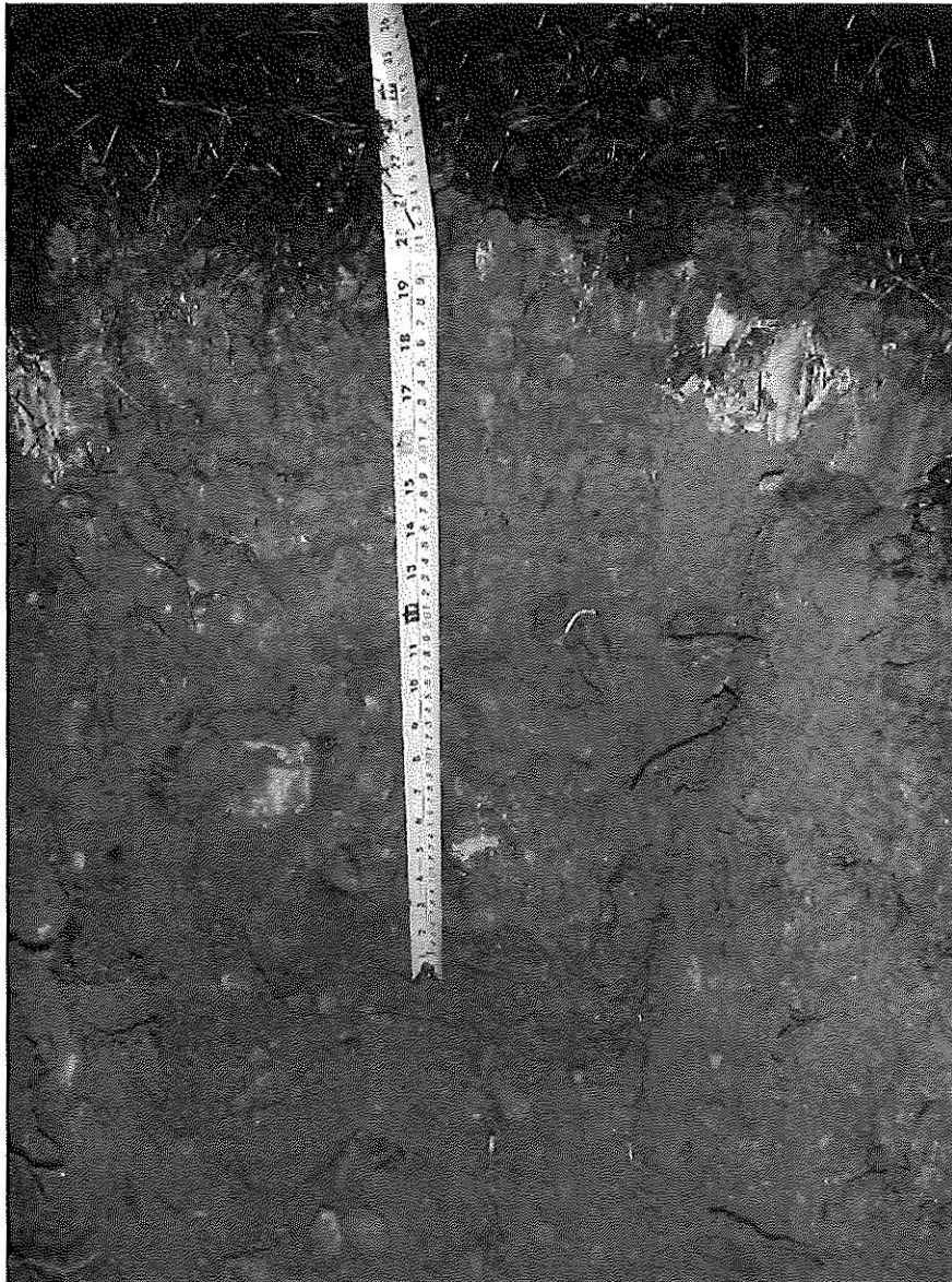
Figure 5-4: Soil profile at the hillslope-scale study site. Note, the poor density of root hairs and a thinner organic layer compared to plot-scale soil profile. The sandy patches indicate locations of lysimeters. (Photo: M Srinivasan, NIWA).
