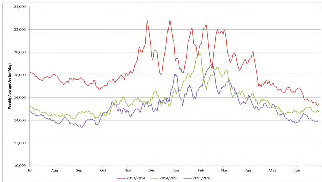
Figure 6 District wide water demand for the last three years has changed with the installation of meters and new metered charging in place
