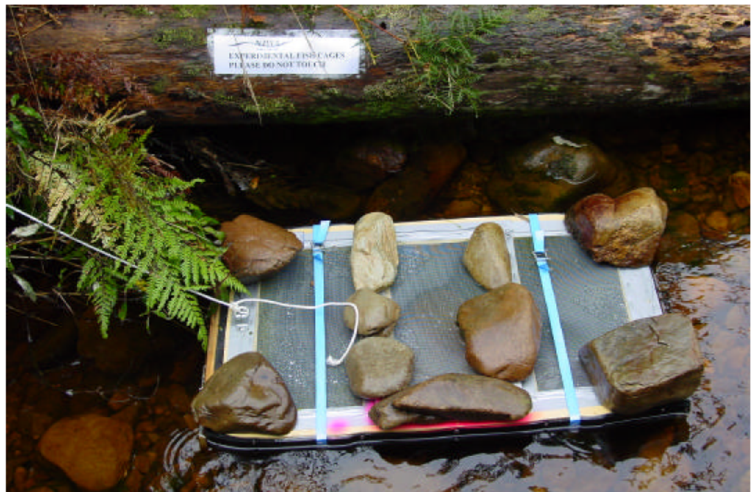
Figure 3: Photo of the experimental fish cages that housed 8 individual fish at sites above and below areas where 1080 baits were added to the streams.
