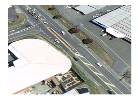
The layout of the current Milne Drive / Kapiti Road junction is shown above. This confirms that the Kapiti Road westbound approach clearly operates as a single lane with a very short flare approaching Milne Drive. The Milne Drive approach is a wide single lane which can be used by two short vehicles if they are correctly positioned but larger or incorrectly positioned vehicles mean that this stop line operates as a single lane entry.
