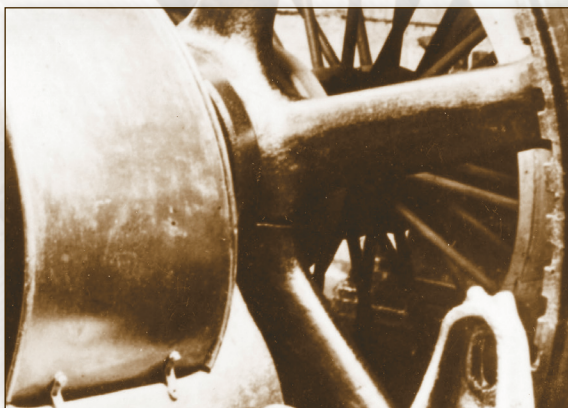
A new suction gas engine working on coal at the Brown's Flax Mill in Waikanae, 1916
