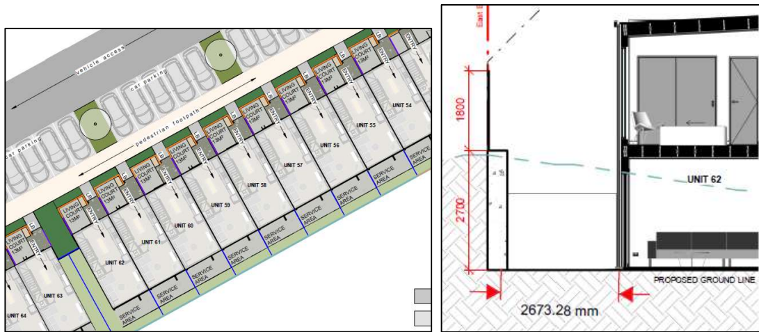
Figure 1: Orientation of private indoor living areas to the south, and disconnected from primary outdoor living court; and extensive retaining at the southeast boundary.
