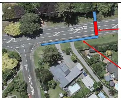
New footpath to be constructed as part of permanent Pedestrian Crossing Point in 2024-2027
