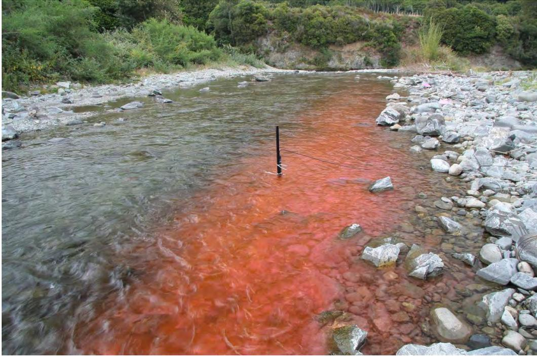
**Figure 3-7: Dye test in Waikanae River**
