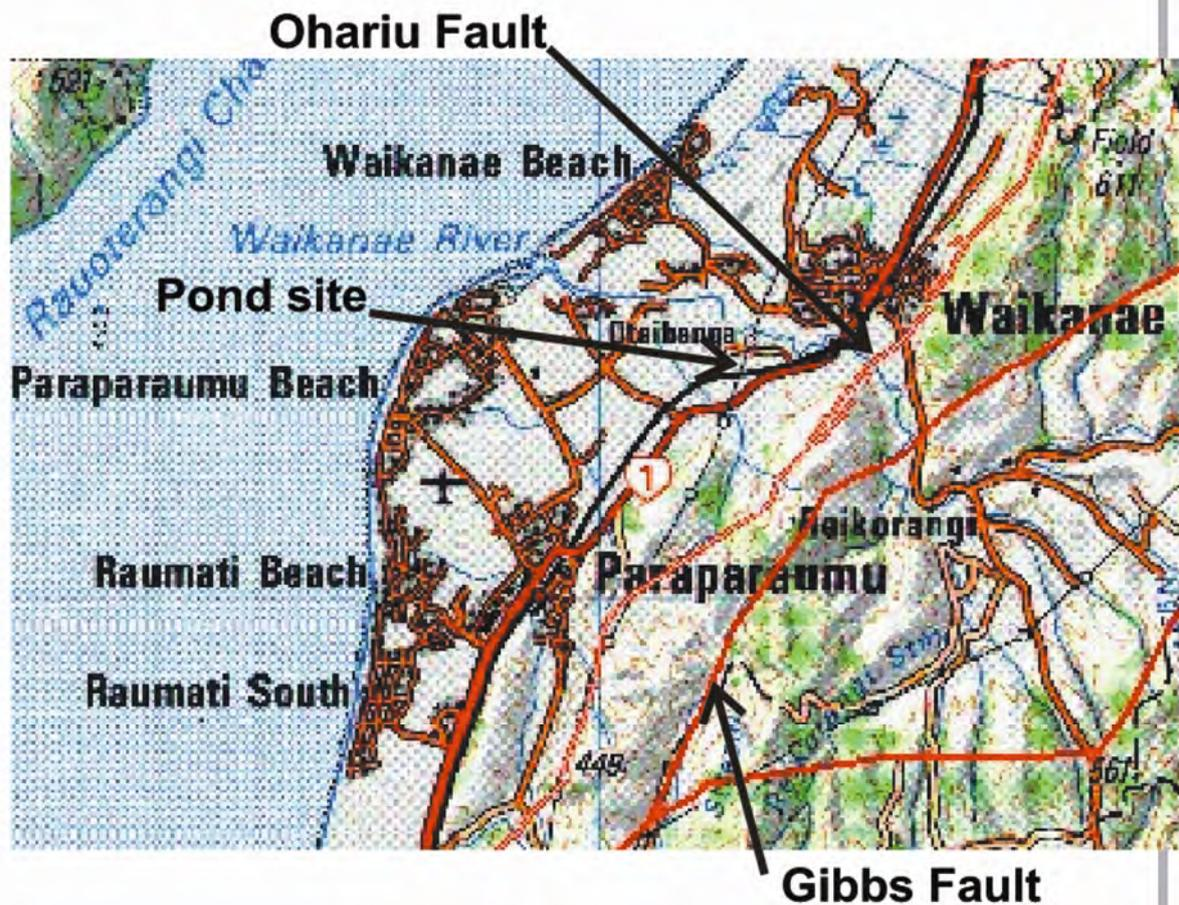
**Figure 7-4: Active Faults in the Vicinity of Storage Pond Site<sup>24</sup>**
