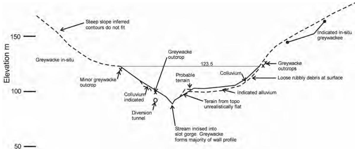
**Figure 5-3: Geologic Profile Along Dam Axis Looking Downstream**
