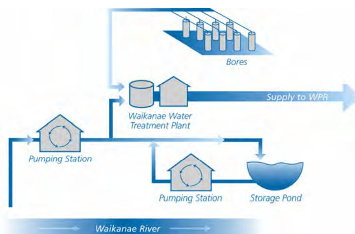
**Figure 7-1: Waikanae Borefield and Storage Option Schematic**
