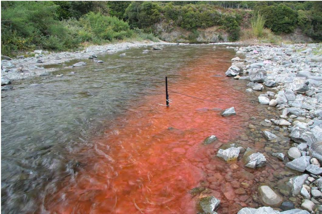
**Figure 3-7: Dye test in Waikanae River**
