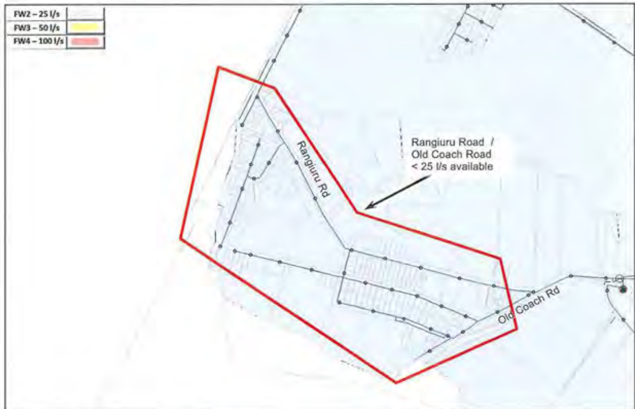
Figure 6-13: Rangiuru Fire Flow Deficiency
