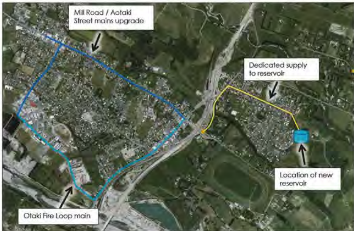
Figure 3-1: Location of new reservoir and configuration of fire loop main
