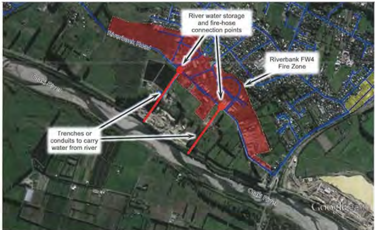
Figure 7-24 : Alternative Riverbank Road Fire Supply - Otaki River
