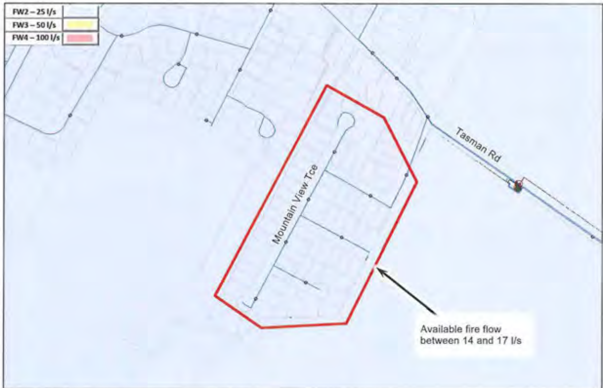
Figure 6-14: Mountain View Terrace Fire Flow Deficiency
