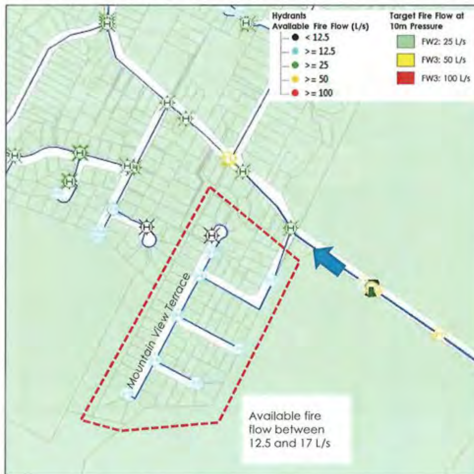
Figure 6-8: Mountain View Terrace fire flow deficiency
