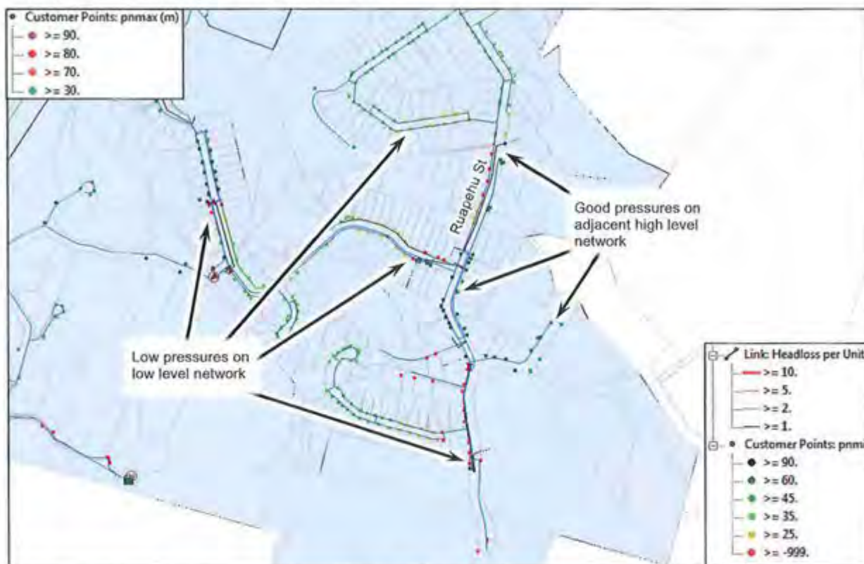
Figure 6-6 : Riwai High Level Pressures – 2046 Non-upgraded
