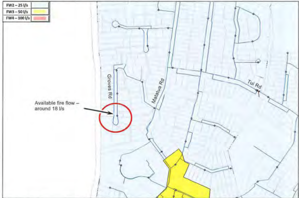
Figure 6-19: Groves Road Fire Flow Deficiency
