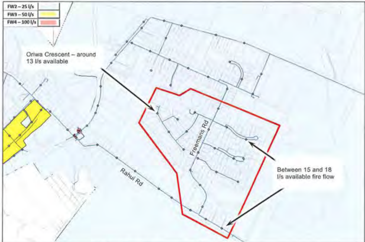
Figure 6-17: Freemans Road Fire Flow Deficiency
