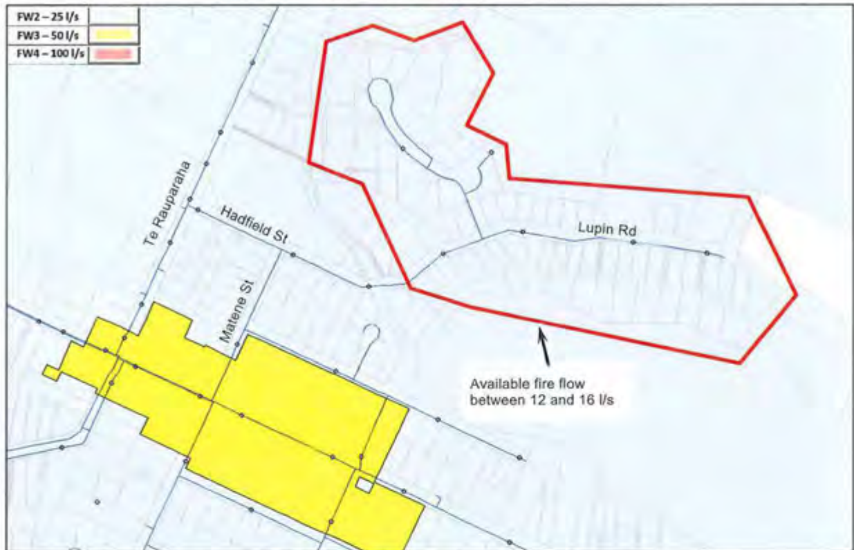
Figure 6-15: Lupin Road Fire Flow Deficiency
