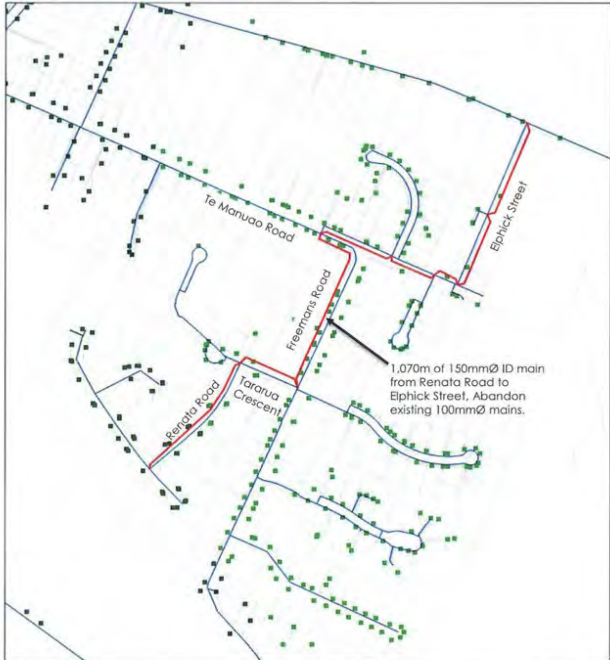
Figure 7-17: Freemans Road fire supply upgrade
