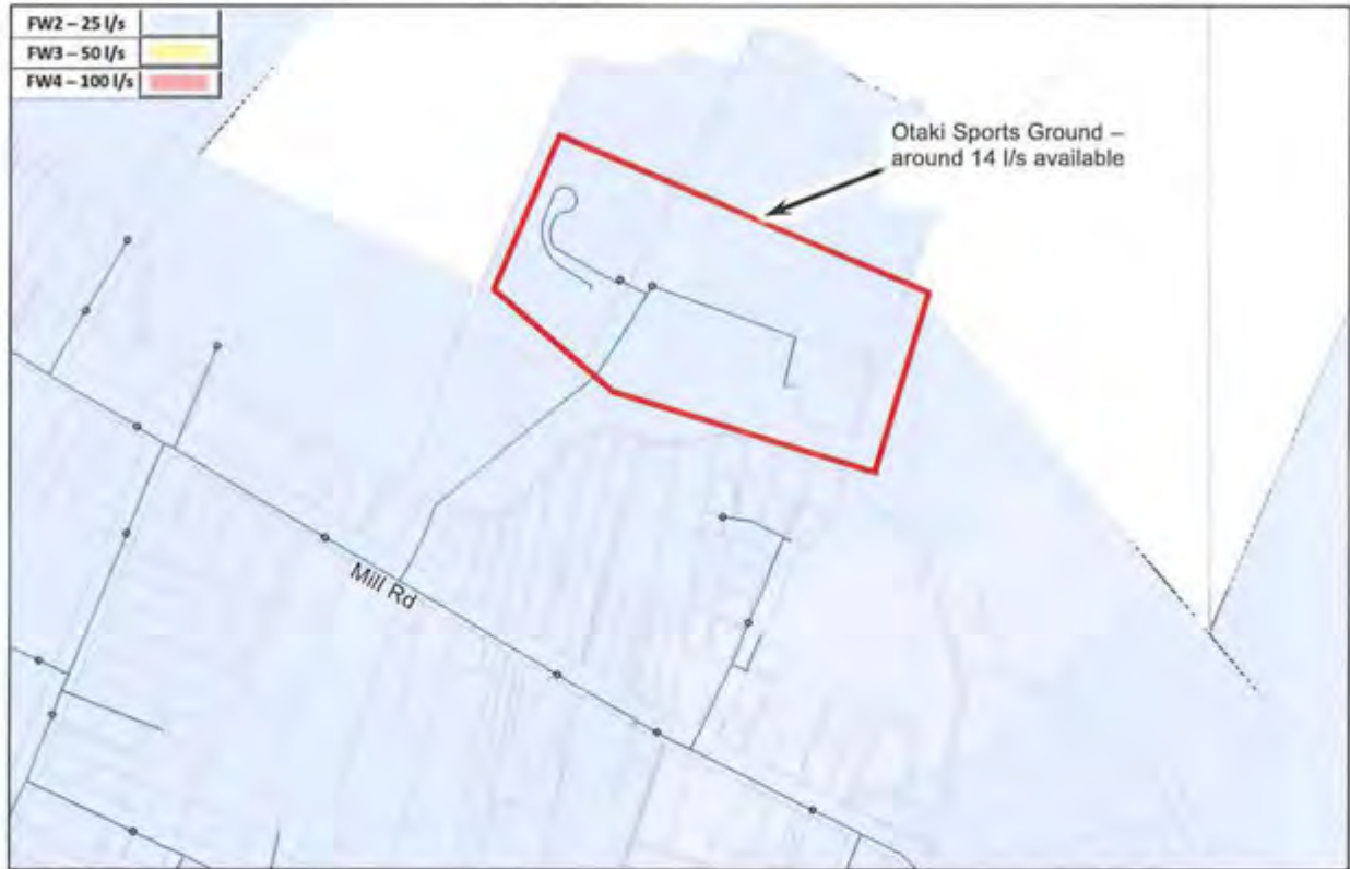
Figure 6-16: Otaki Sports Ground Fire Flow Deficiency
