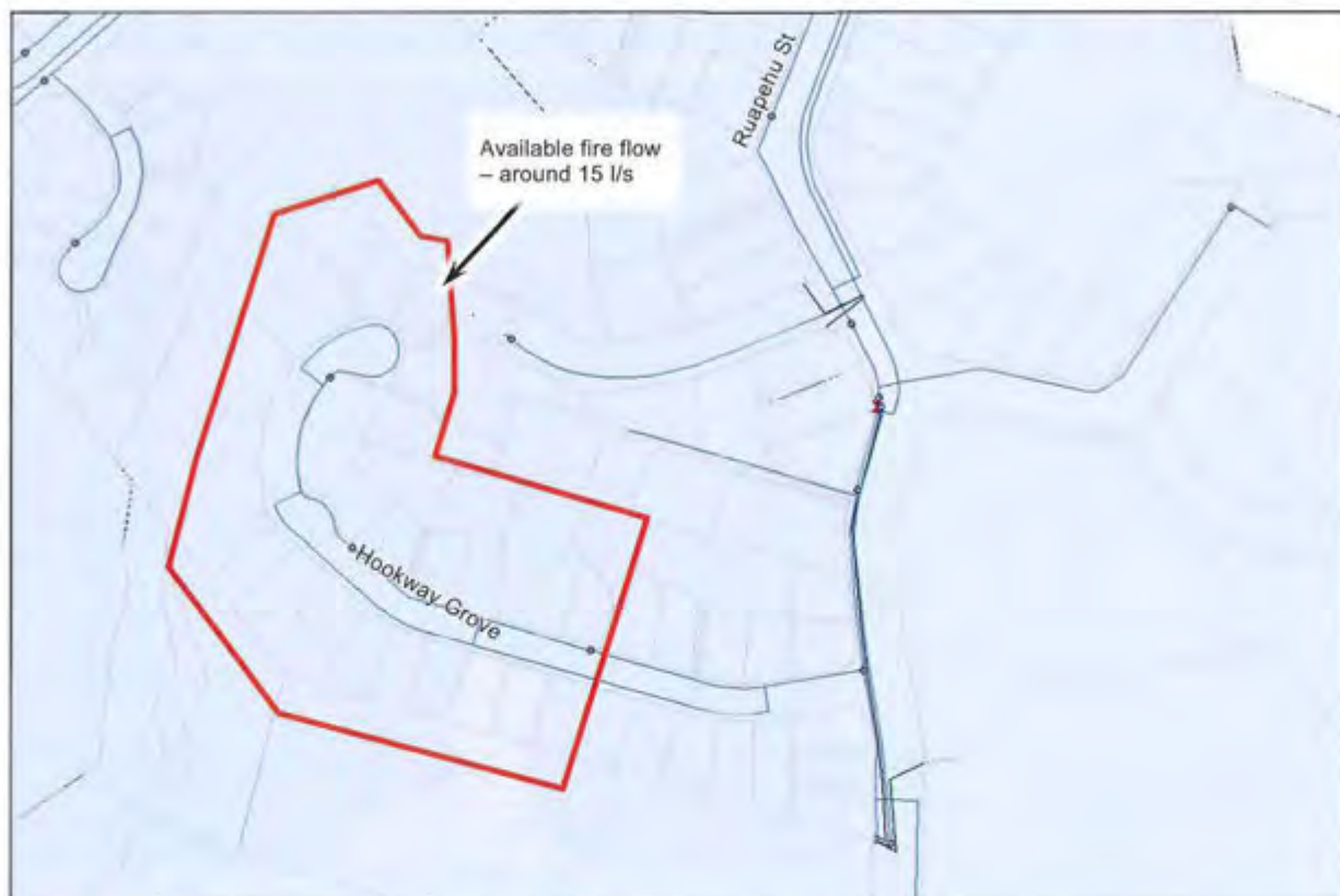
Figure 6-20: Hookway Grove Fire Flow Deficiency
