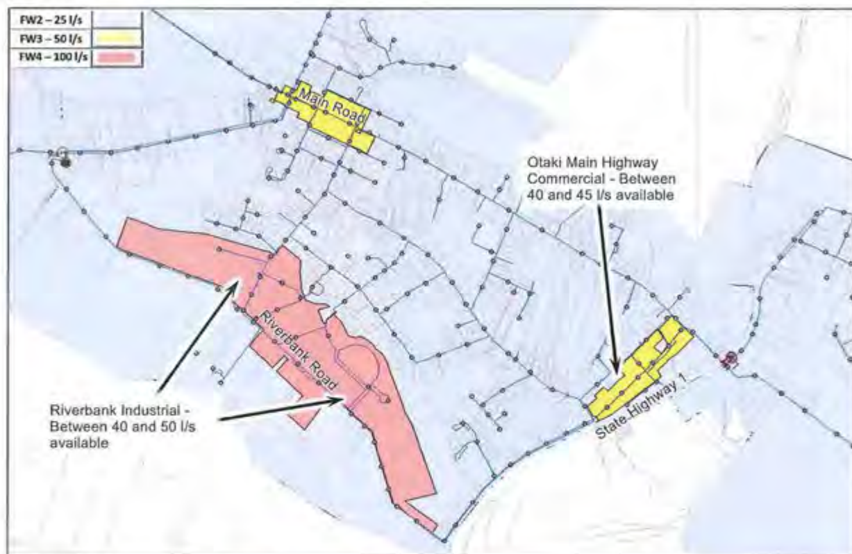
Figure 6-10: Riverbank Road and Otaki Main Highway Fire Flow Deficiency
