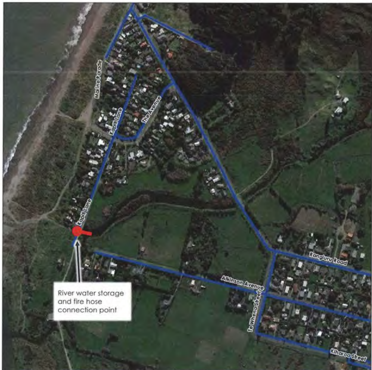
Figure 7-11: Alternative Rangiora fire supply option
