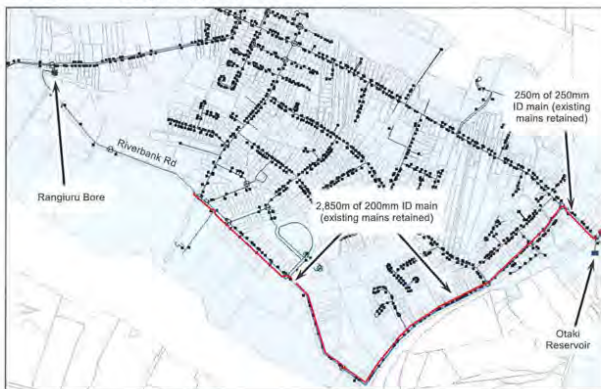
Figure 7-23 : Otaki Loop Fire Main
