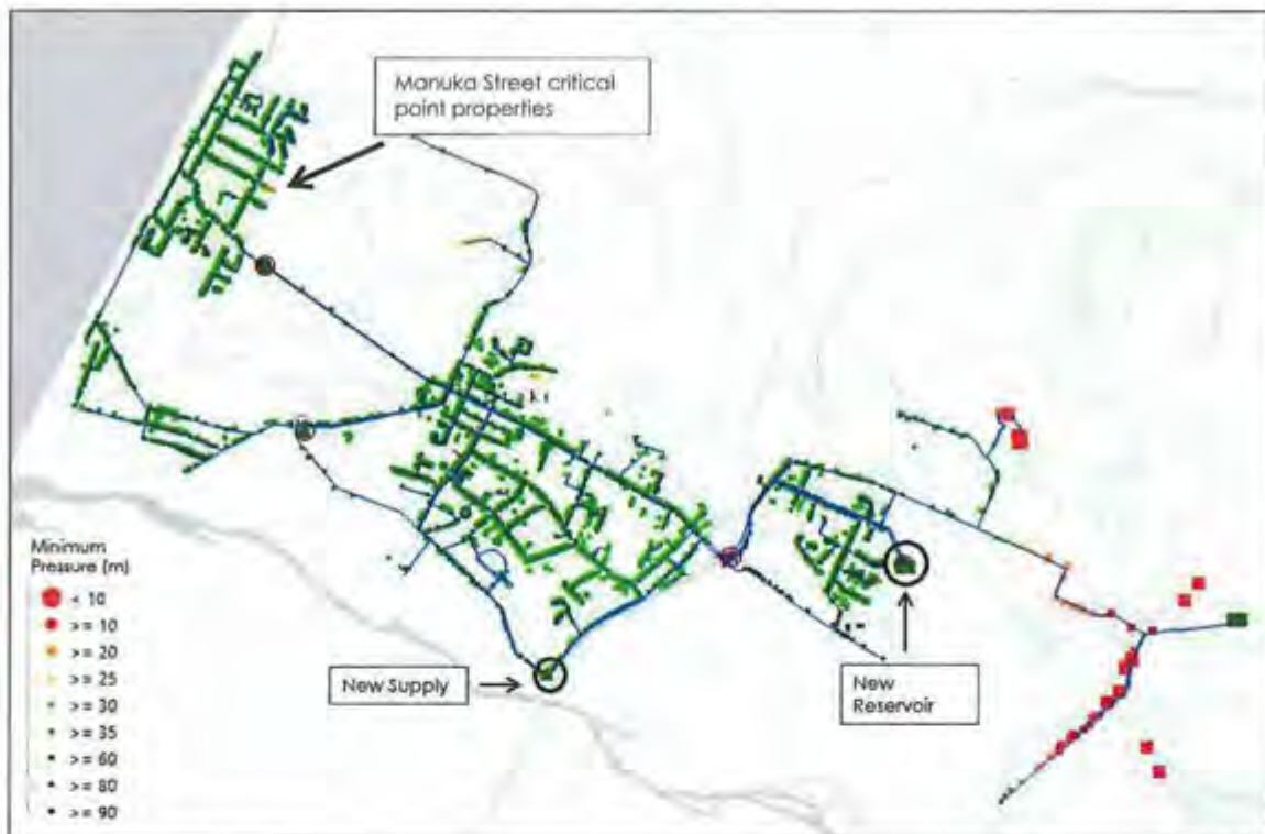
Figure 4-2: Current peak day pressure (m) with Tasman and Rangiuru out of commission
