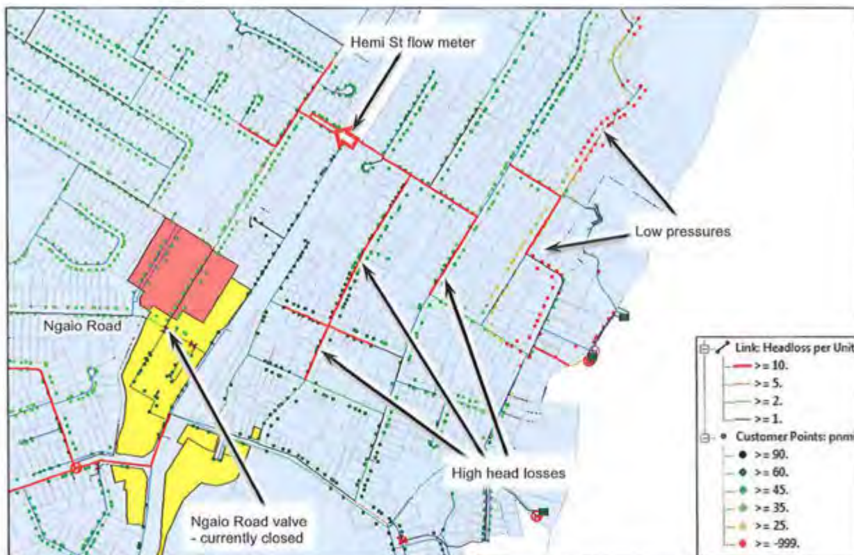
Figure 6-5 : Hemi Street DMA, Tui Crescent and Kotare Street Pressures - 2046 Non-upgraded
