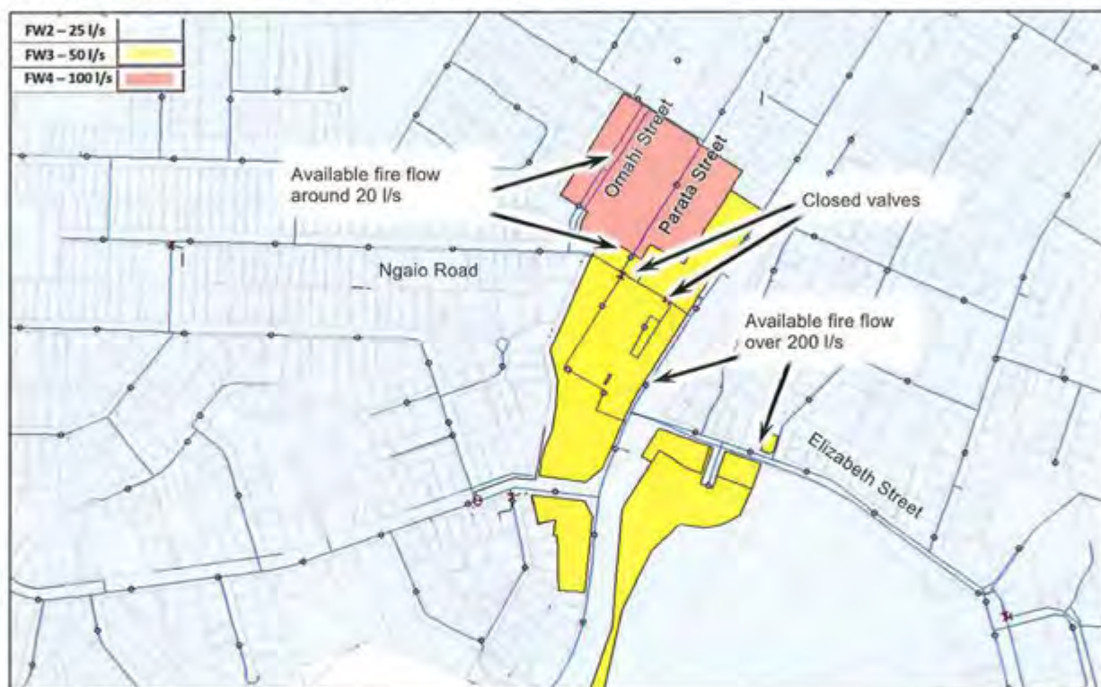
Figure 6-9 : Waikanae Town Fire Flow Deficiency
