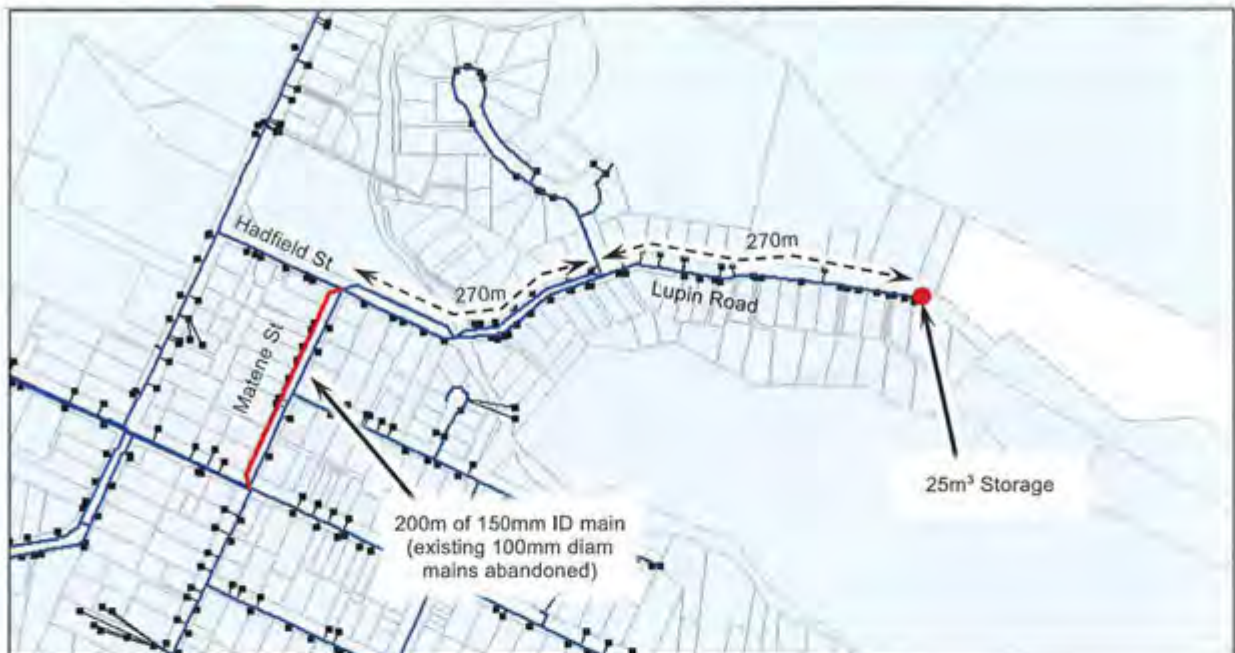
Figure 7-31 : Lupin Road Alternative Fire Upgrade - Storage
