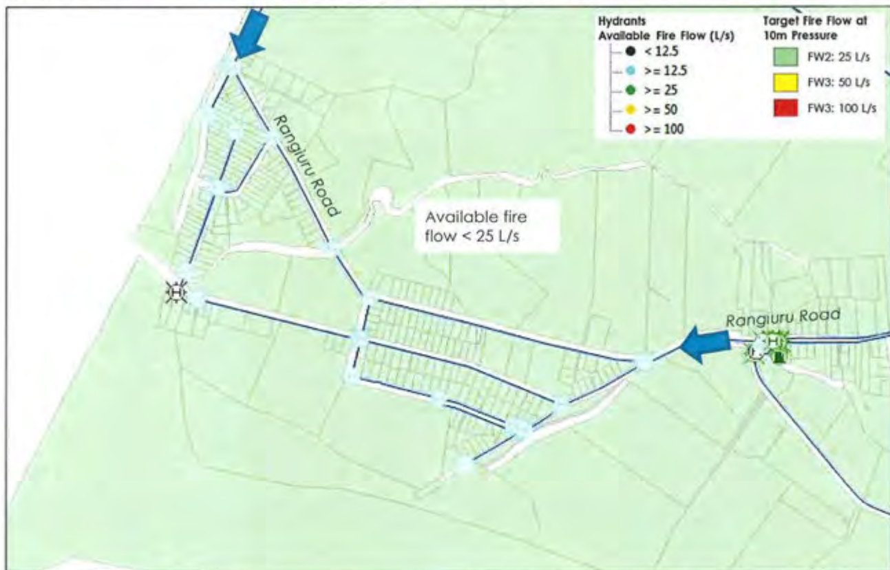
Figure 6-7: Rangluru fire flow deficiency
