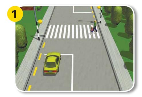
It takes an alert driver 1.5 seconds to react to a pedestrian to a pedestrian brake. In that time, at brake. In that time, at 50km/h, a car covers 21 metres on the road.
