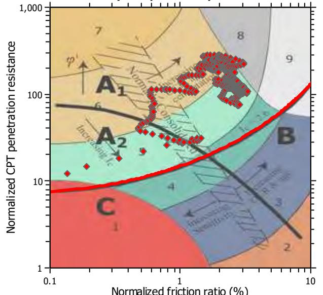
Zone A<sub>1</sub>: Cyclic liquefaction likely depending on size and duration of cyclic loading
