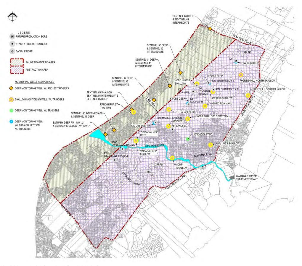
Figure 2: Location Plan – Waikanae Borefield Abstraction Wells and Monitoring Bores
