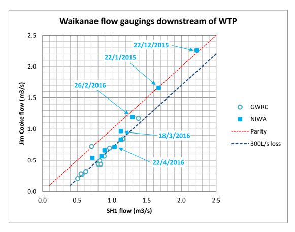
Figure 5: Waikanae River Flow Gaugings near SH1 and Jim Cooke Park
