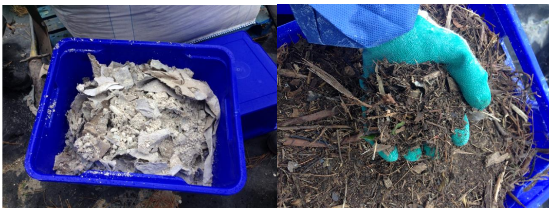
Figure 1. Crushed plasterboard and greenwaste
