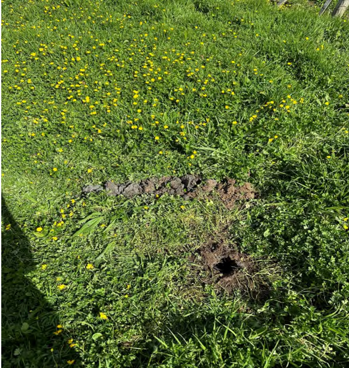
Photo 3 – Augered hole approximately 0.85m below GL showing saturated loose to dense sand with dark waterlogged clay found at the base
