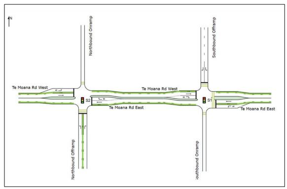
Figure 2 - Layout of Te Moana Rd/Kapiti Expressway Interchange - Source (SIDRA)
