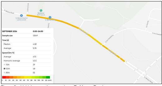
Figure 6 – Vehicle operating speeds on Te Moana Road.
