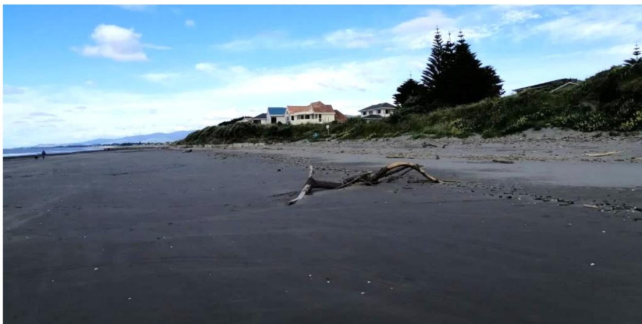
Figure 7.2: Paraparaumu Beach near Ngapotiki Street access (south side of cusplate foreland apex) showing vegetated dune elevations in the order of 6 – 6.5 m. Note the seaward location of the houses at 175-177B Manly Street and the small block seawall feature at the toe of the dune in front of these houses.
