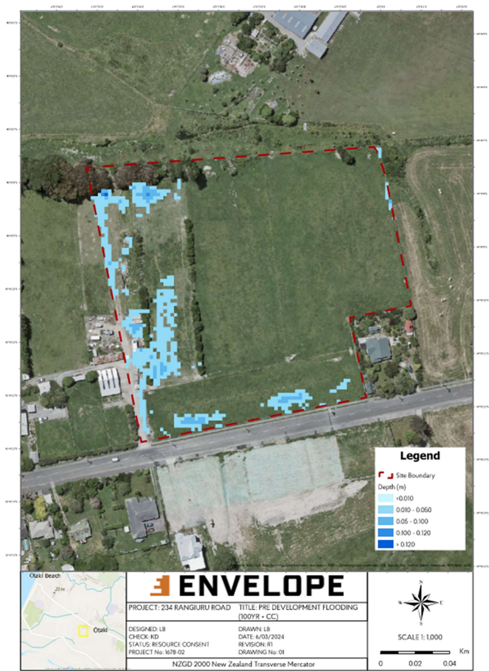
Figure 2. Updated pre-development flood model results from KCDC Model.
