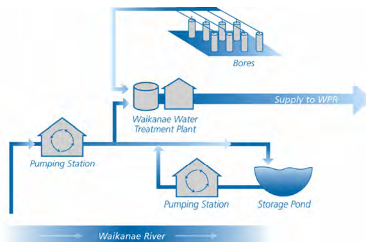
Figure 7-1: Waikanae Borefield and Storage Option Schematic
