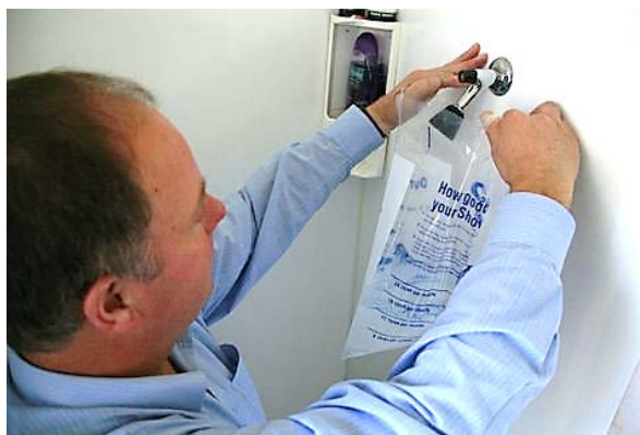
The Ecodesign Advisor demonstrates how to test the flowrate with a Council shower bag
