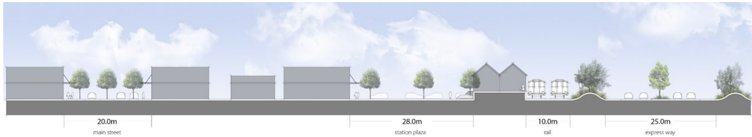
Otaki cross section for Main Street through to Expressway
