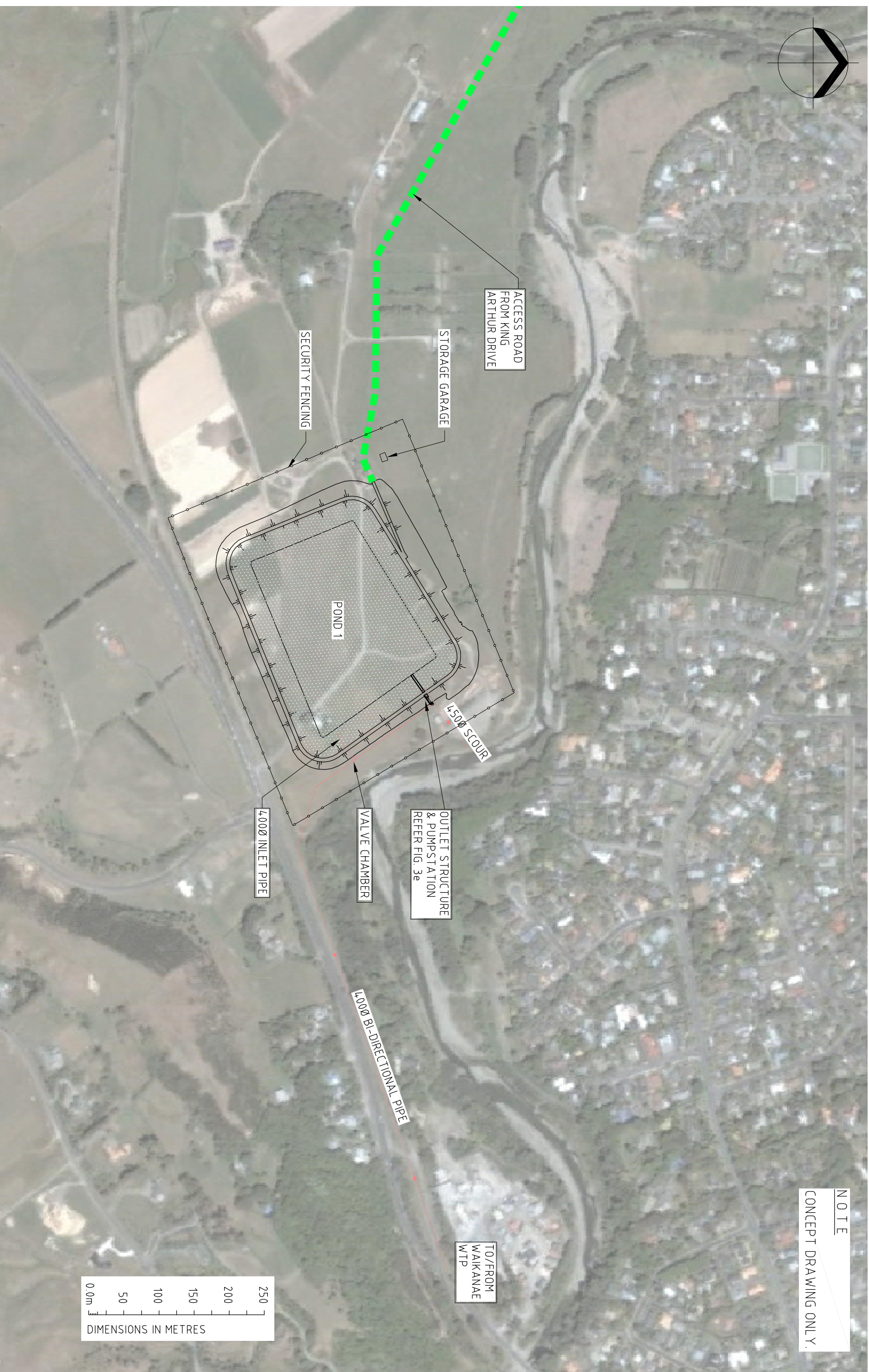
OPTION D1-2 - BOREFIELD & STORAGE STORAGE POND
