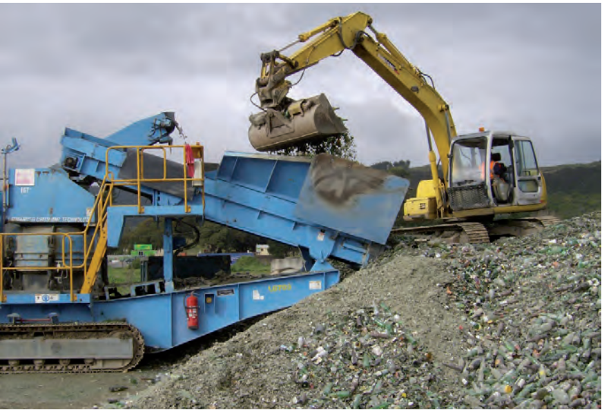
Glass crushing at the Otaihanga Landfill, for use in the gas-venting layer for the final cap on the landfill.
