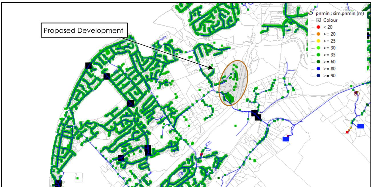
Figure 4-1: Minimum pressures in the WPR network after development (Current Peak Day)
