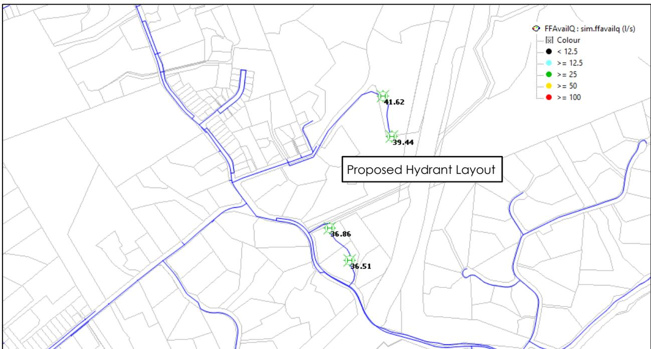
Figure 4-3: Available Fire Flow at hydrants with development (Current Peak Day)
