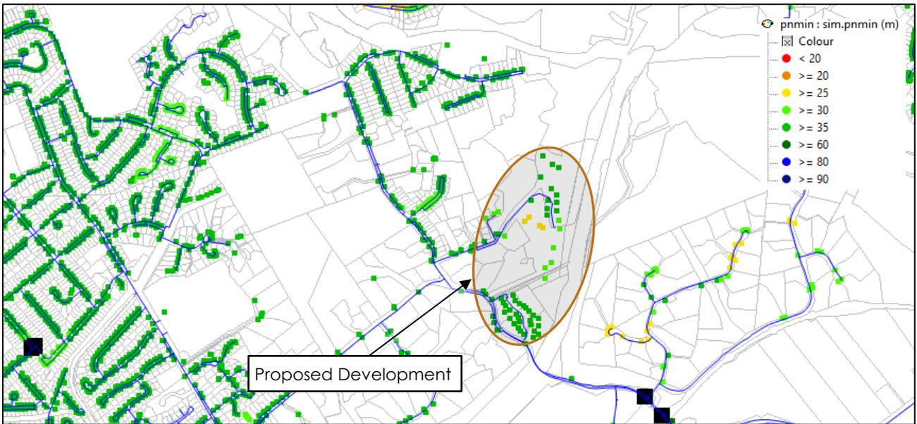
Figure 4-4: Minimum pressures in the WPR network after development (Future Peak Day)
