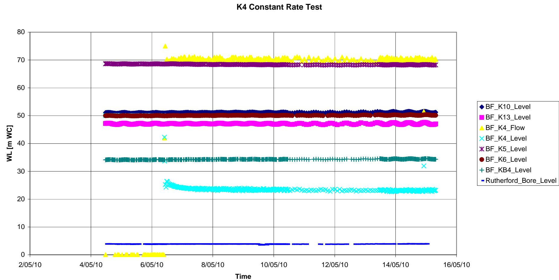
**Relative water levels and pump rate during K4 constant rate test**
