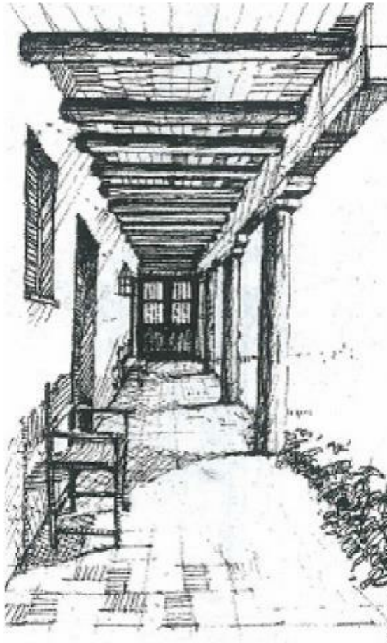
Figure 54: Utilisation of eaves and porches to manipulate solar gain and loss
